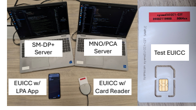
Figure 10: ZK-eSIM Implementation and Evaluation Testbed
