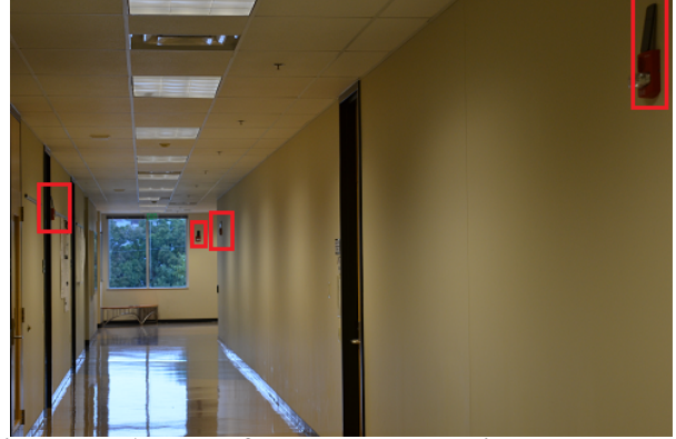
Figure 7: A part of the testbed showing smartphones (hanging near the fire alarms) that served as gateways.
