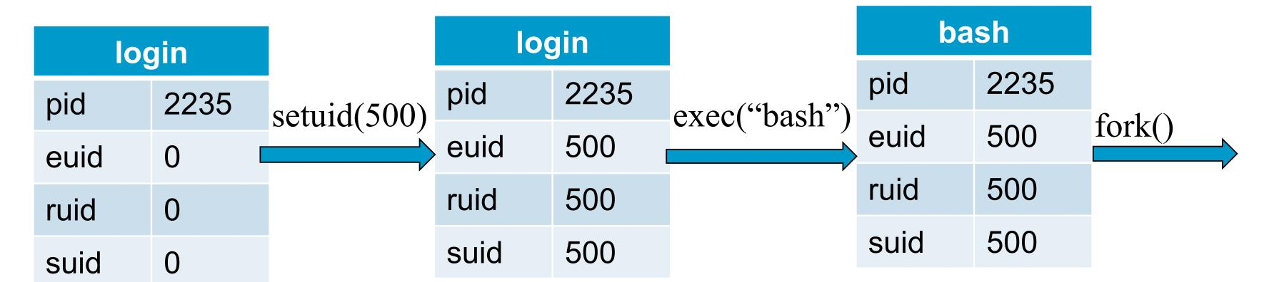
After the login process verifies that the entered password is correct, it issues a setuid system call.
